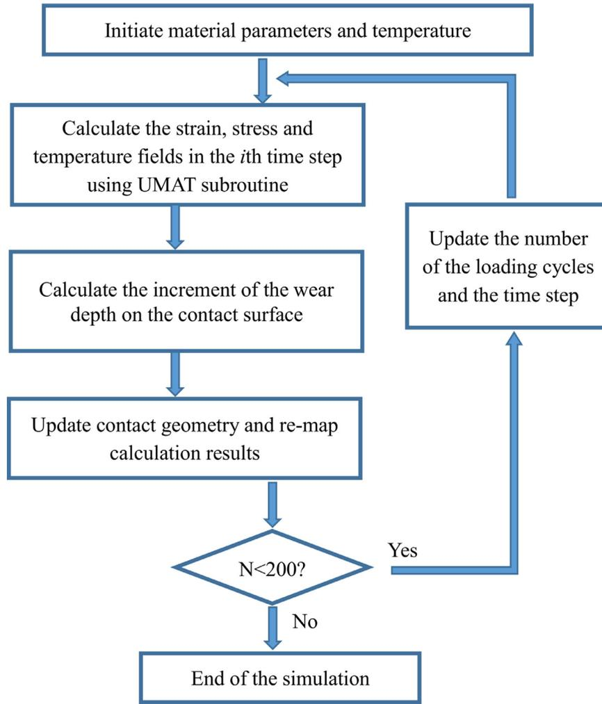
Fig. 4. Simplified flowchart of the numerical implementation.
