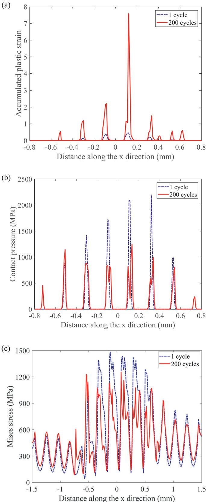
**Fig. 7.** Distributions of (a) the accumulated plastic strain, (b) the contact pressure, and (c) the Mises stress on the rough surface of the specimen for the simulation case with  $R_a = 12.5 \mu\text{m}$ .
