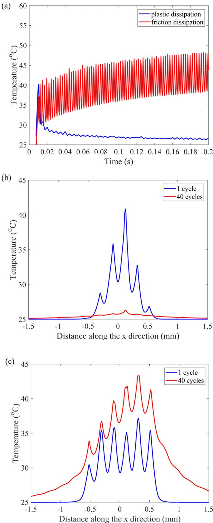
**Fig. 8.** (a) Evolutions of the temperature on the rough surface of the specimen obtained by two approaches considering the plastic dissipation and the friction dissipation respectively. Distributions of the temperature on the rough surface under the condition of considering only (b) the plastic dissipation and (c) the friction dissipation.
