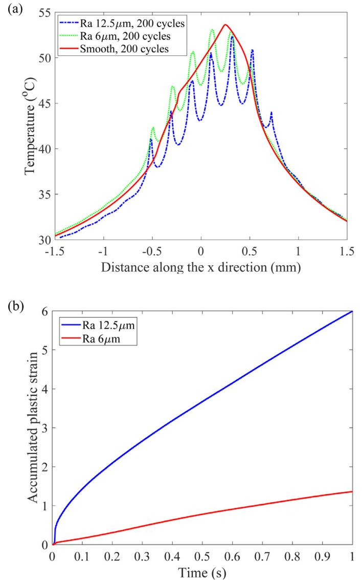
**Fig. 9.** (a) Distributions of the temperature on the contact surfaces after 200 cycles under the three conditions of surface roughnesses. (b) Evolutions of the accumulated plastic strain at the maximum temperature points on two rough surfaces.
