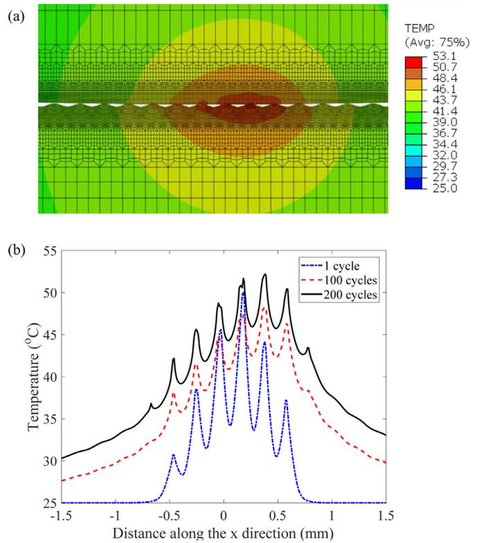
Fig. 5. (a) Temperature field in the contact zone after 200 cycles for the simulation case with  $R_a = 12.5 \mu\text{m}$ . (b) Distributions of the temperature on the rough surface of the specimen after 1, 100 and 200 cycles.
