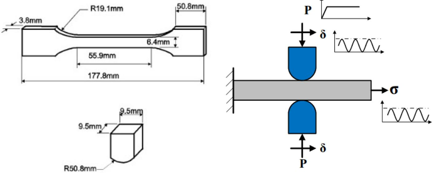
Fig. 1. Schematic diagram of the fretting contact configuration.
